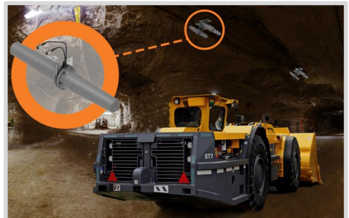
2x HELI-19 antennas mounted on the BRKT-45 for MIMO application
